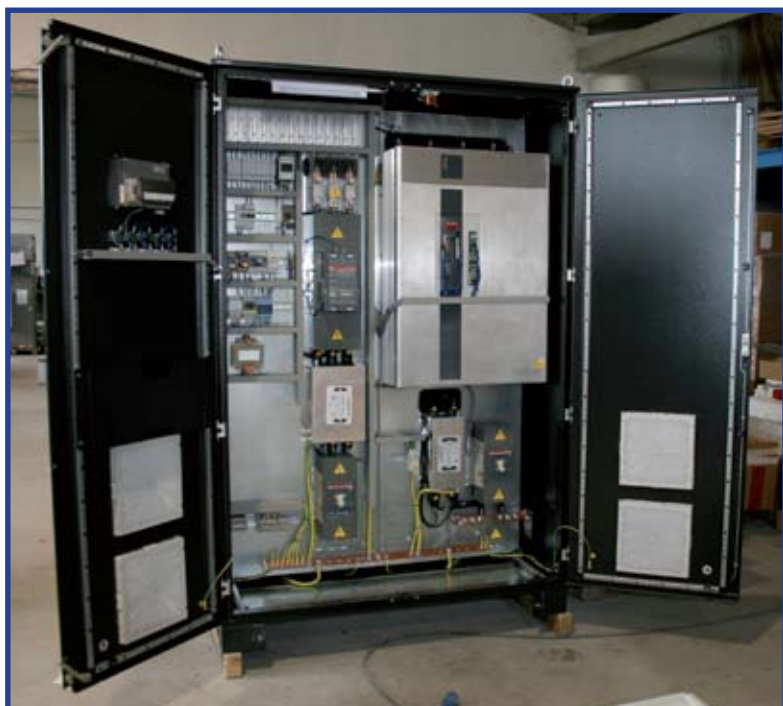
Interno Inverter FAI FPV250
